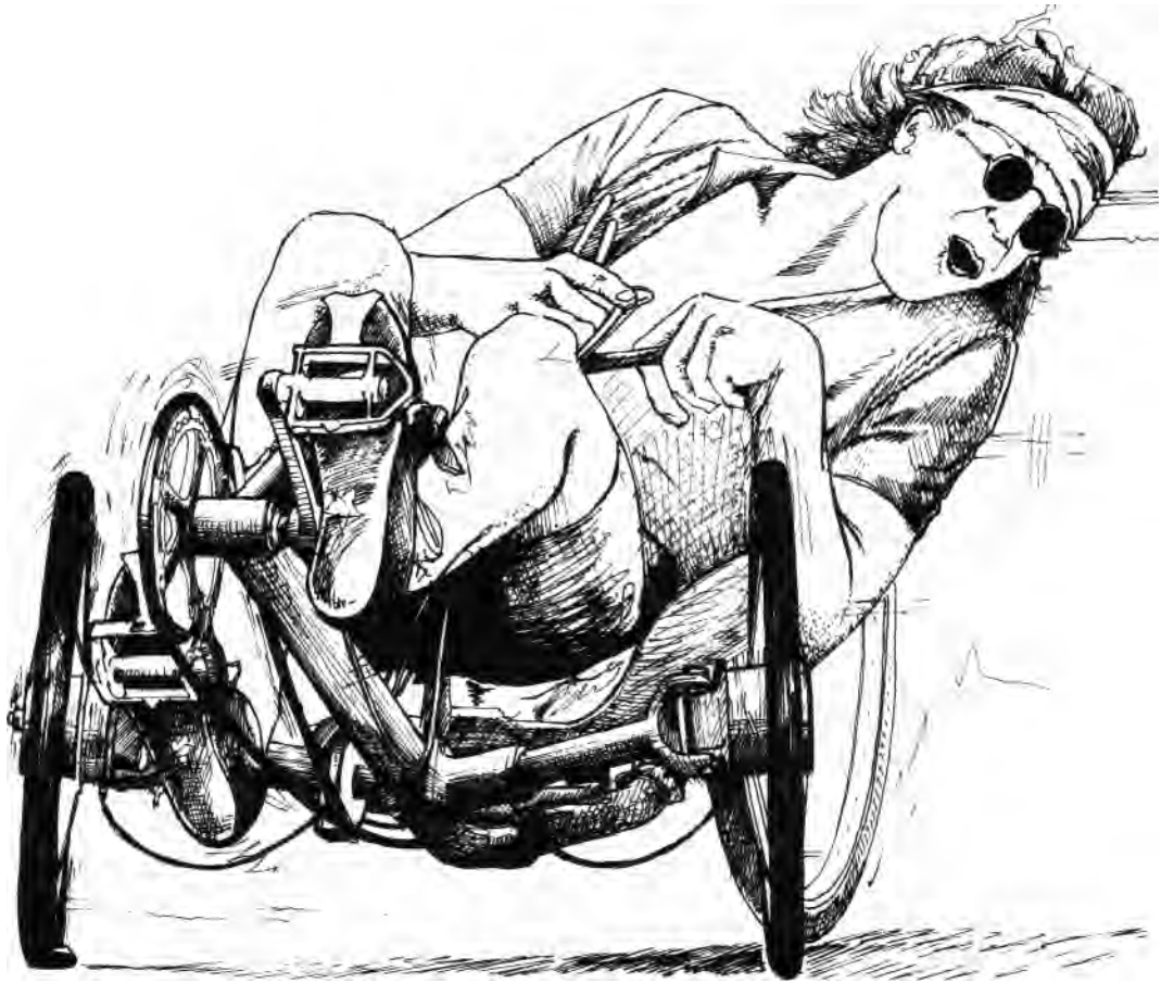
Andy Pegg riding an early Speedy. When cornering hard, with a trike, it is essential to lean to the inside - note stress to tyres.
