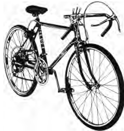
Classic 10-speed: American Columbia with 'gut-ripper' gear shift lever talons and 'suicide' dual brake levers.
