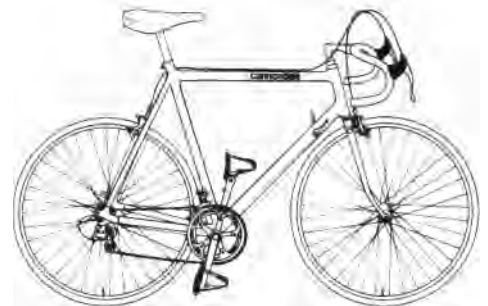
Cannondale Black Lightning (1987) with oversize aluminium frame tubes; light, stiff, fast, and affordable.
