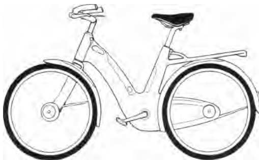
Concept study for a monocoque city bike with cantilever wheels and enclosed chainguard,
